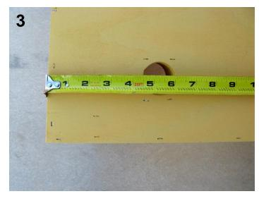
Now let's find the *vertical position* of hole centers: measure the distance from the bottom edge of the wall to the center of each entrance hole:
