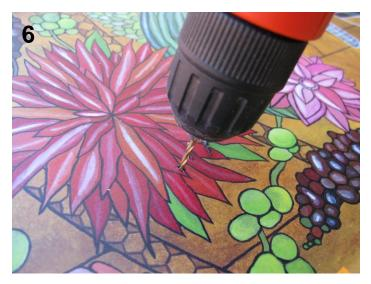
Take a piece of scrap plywood or wood at least 3/8" thick. Drill a pilot hole with the pilot bit of your hole saw. [9] (Try to drill as square to the surface as you can.) Predrill the pilot hole in the art panel and the board under it with the pilot bit of your hole saw [8]. (Don't let the hole saw
